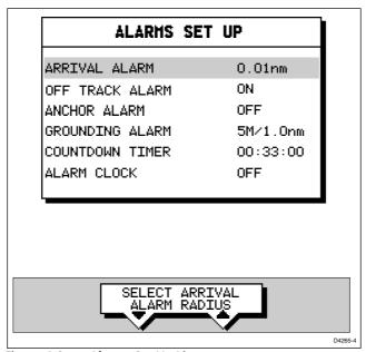
Figure 4-2: Alarms Set Up List
